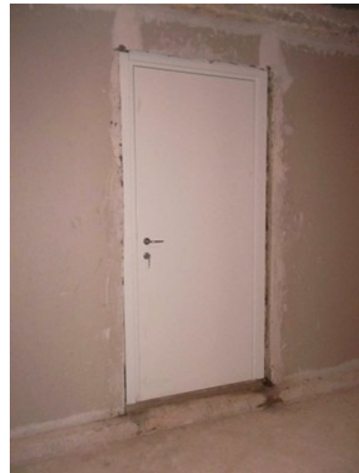
Left: Finishing of the door leaf at Valsecchi's premises. Right: Set-up of the door prototype at AIMCM for the acoustic tests.
